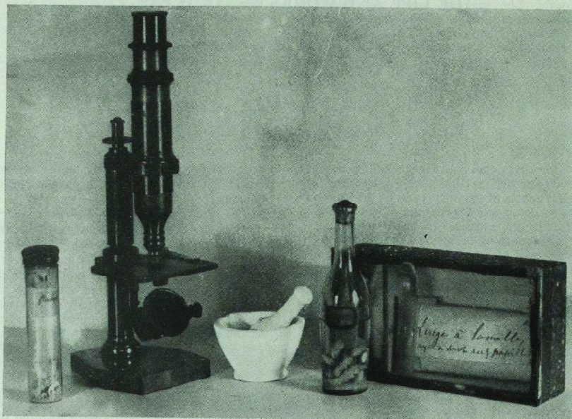
The apparatus used by Pasteur in his studies on the diseases of silkworms. It consists of a collecting bottle, a microscope, a pestle and mortar for grinding up the moths or eggs to see if corpuscles are present, a bottle to convey dead moths in brandy to the local research centre. A box containing the cloth in which the eggs and moths of one year are wrapped is also shown. These eggs and moth are kept for investigation next year in order to produce healthy cocoons.
