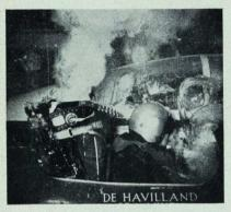
1962 Aircraft Underwater Escape Trials. Ejecting at 20 ft. beneath the surface from the observer's compartment in a Sea Vixen, using the prototype automatic underwater escape system.
