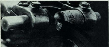
Above: Sawing a diamond. Right: Polishing the facet of a diamond.
