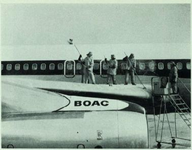
Chemical washdown of a Jet Aircraft to remove Radioactive Fallout Debris
