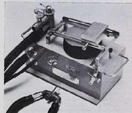
Figure 7. Manley ventilator with bellows and weight above. At left are, from below upwards, gas inlet tube and inspiratory and expiratory tubes. Lower centre is Y-piece for connection of inspiratory and expiratory limbs to patient.
