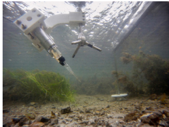
Eddy covariance system measuring river metabolism in the River Ebbles.
