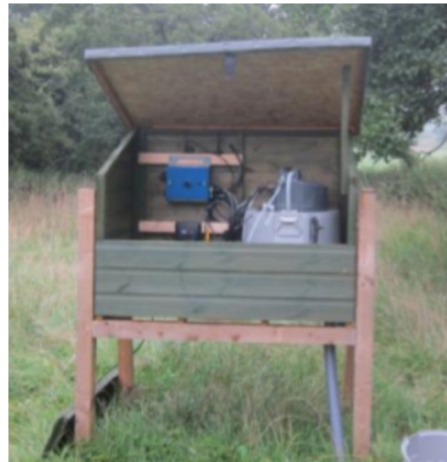
Piezometers to measure direction of water movement and water samplers next to the River Sem.
