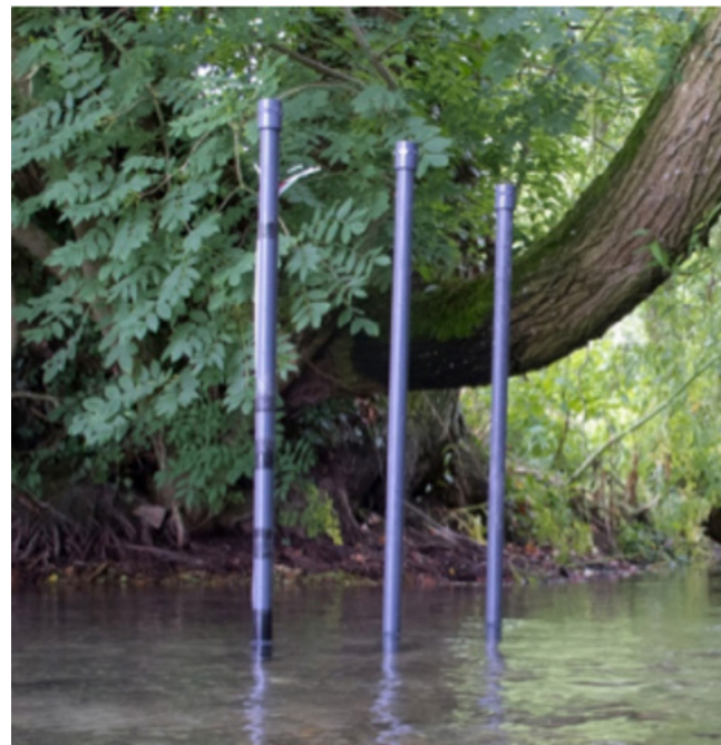
Piezometers to measure direction of water movement and water samplers next to the River Sem.
