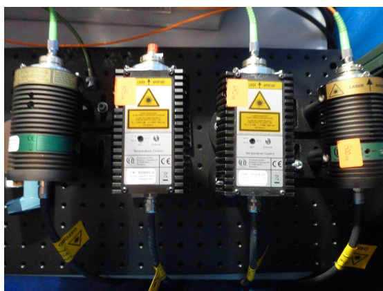
Figure 4.3: The four SMELLIE single-wavelength laser heads.
