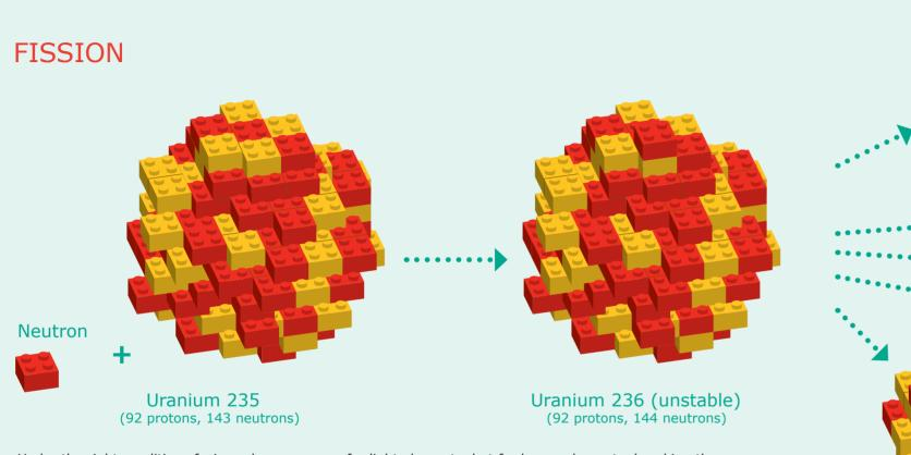
Under the right conditions fusion releases energy for light elements, but for heavy elements, breaking them up releases energy. In nature, most heavy elements only lose a small fraction of their protons and neutrons - through alpha radiation. However, there are some elements which will split into two large parts, if we fire a neutron at them. In many nuclear power stations, neutrons are fired at an isotope of uranium (uranium-235).
